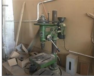
Photo of non-conformity NC-The drilling machine was not equipped with belt guard.JPG
