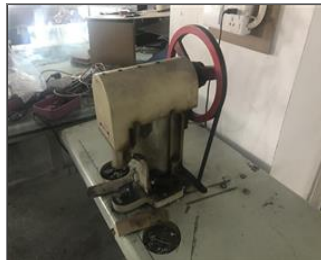
Photo of non-conformity NC-The button attaching machine was not equipped with guard circle and belt guard.JPG
